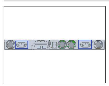
Start up your system by connecting the power cables
