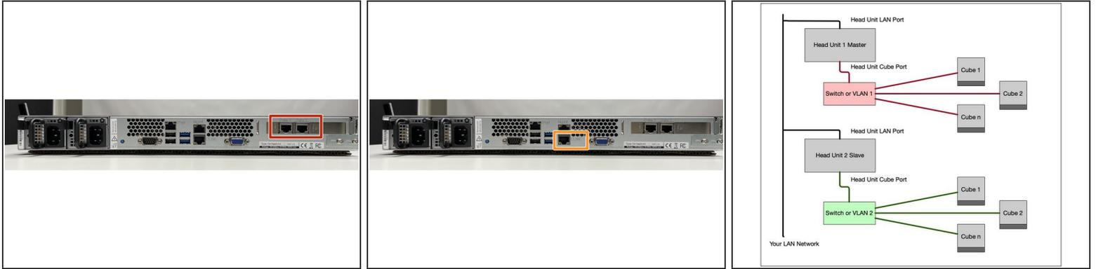
⚠ The network connections on the head units are pre-assigned and must not be swapped.
