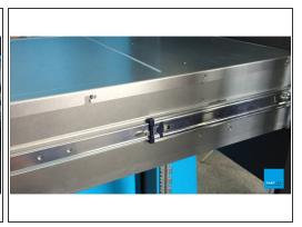
Slide G5000 Controller halfway into the Rack, until the lever on the inner arm latches
