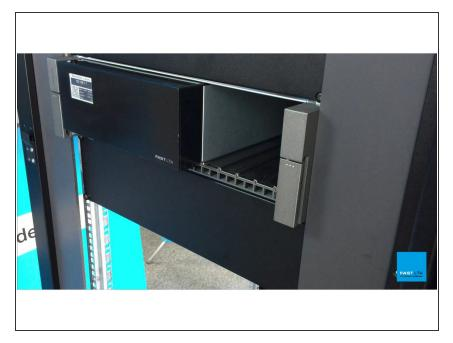
Gently push G5000 Controller into the Rack until both Rack Flanges have latched
